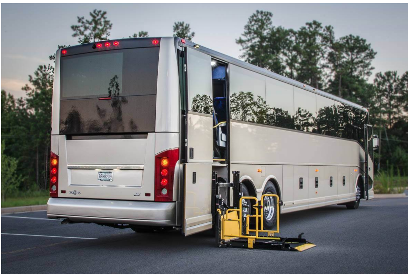
Figure 20. Van Hool C2045 Motor Coach with ADA Lift
