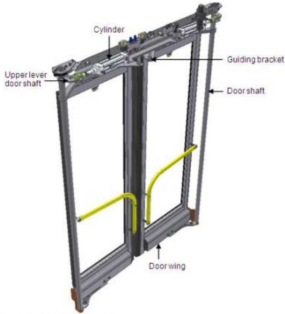
Figure: Door system description
